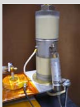
Fig 1. Bench-scale electroporation apparatus used for this study.
